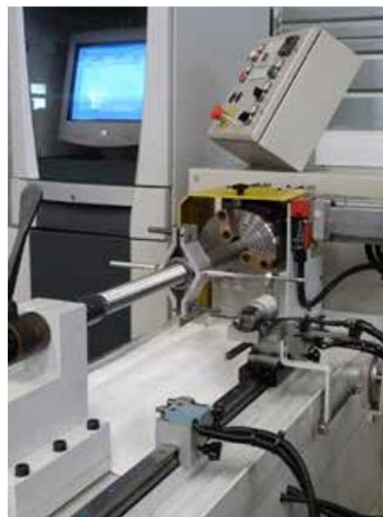
Preload torque test bench
